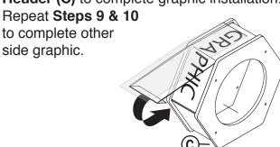
(11) Lower Header (C) onto tower assembly as shown to the left.
