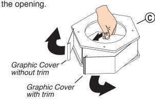
9 Turn **Header (C)** so side *without* trim is up as shown below. Keep other end of graphic cover hooked into header. Slide graphic under graphic cover until end of graphic is butted to the bend of tab at other end of cover.
