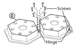
Remove Hinge Pins, from Hinges, flip Bases (D) back over.
