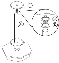
Install lower (9) Wings (H). Hook bottom (longer) prongs into the bottom Hub (I), then tilt up and hook upper prongs into middle Hub (I).
