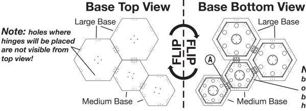
**Note:** The Medium base hinge holes are offset so bases must be rotated until holes align.
