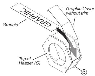
Hook graphic cover tab back into slot on **Header (C)** to complete graphic installation.
